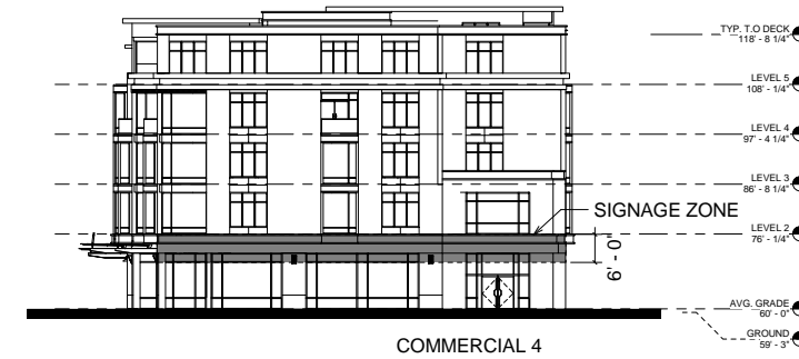
④ COURTYARD ELEVATION 3 - SIGNAGE 1/16" = 1'-0"
