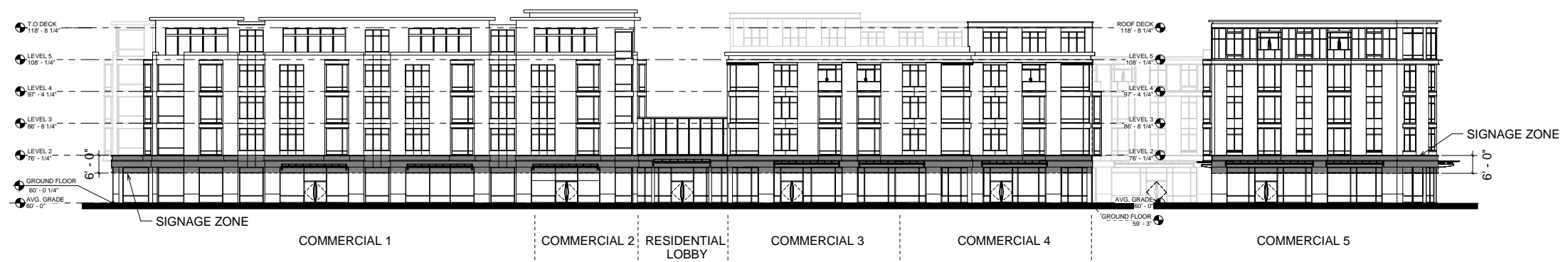
① SOUTH ELEVATION - WASHINGTON STREET - SIGNAGE 1/16" = 1'-0"
