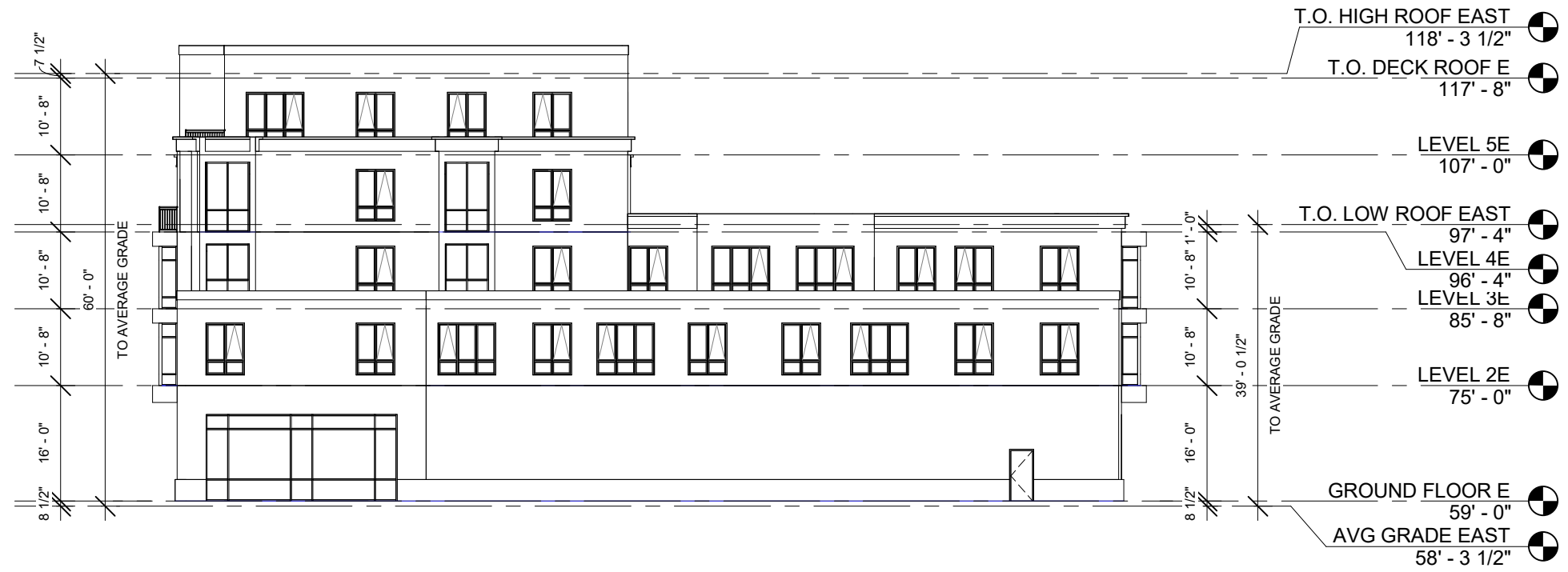
1 EAST BUILDING NORTH ELEVATION 3/64" = 1'-0"
