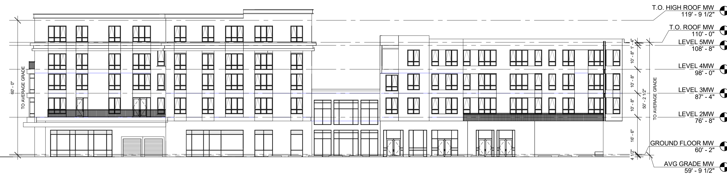
1 WEST/MIDDLE BUILDING NORTH ELEVATION 3/64" = 1'-0"
