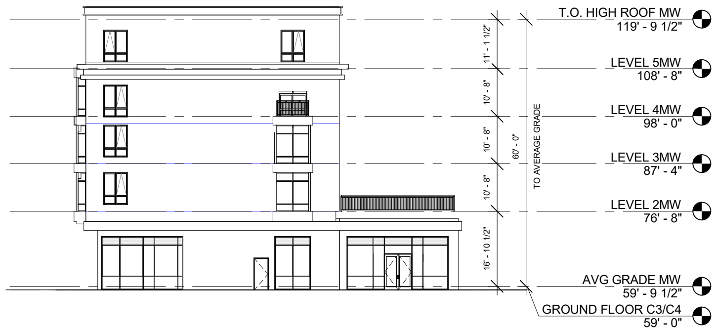
1 MIDDLE BUILDING EAST ELEVATION 3/64" = 1'-0"
