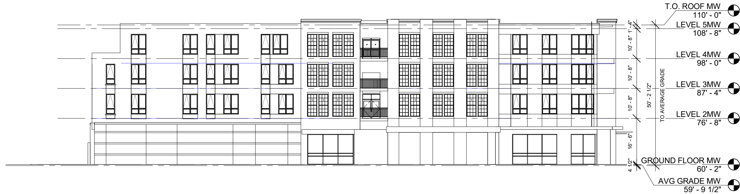
1 WEST BUILDING WEST ELEVATION 3/64" = 1'-0"
