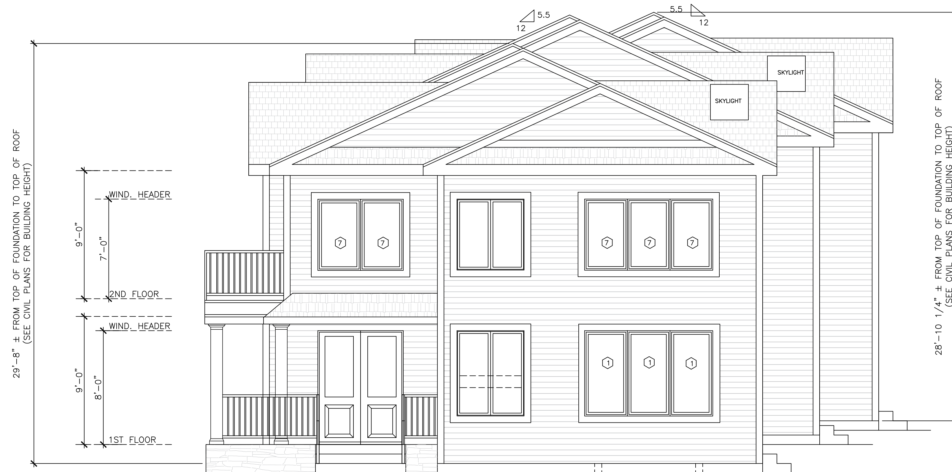
FRONT ELEVATION FOR UNIT 1
