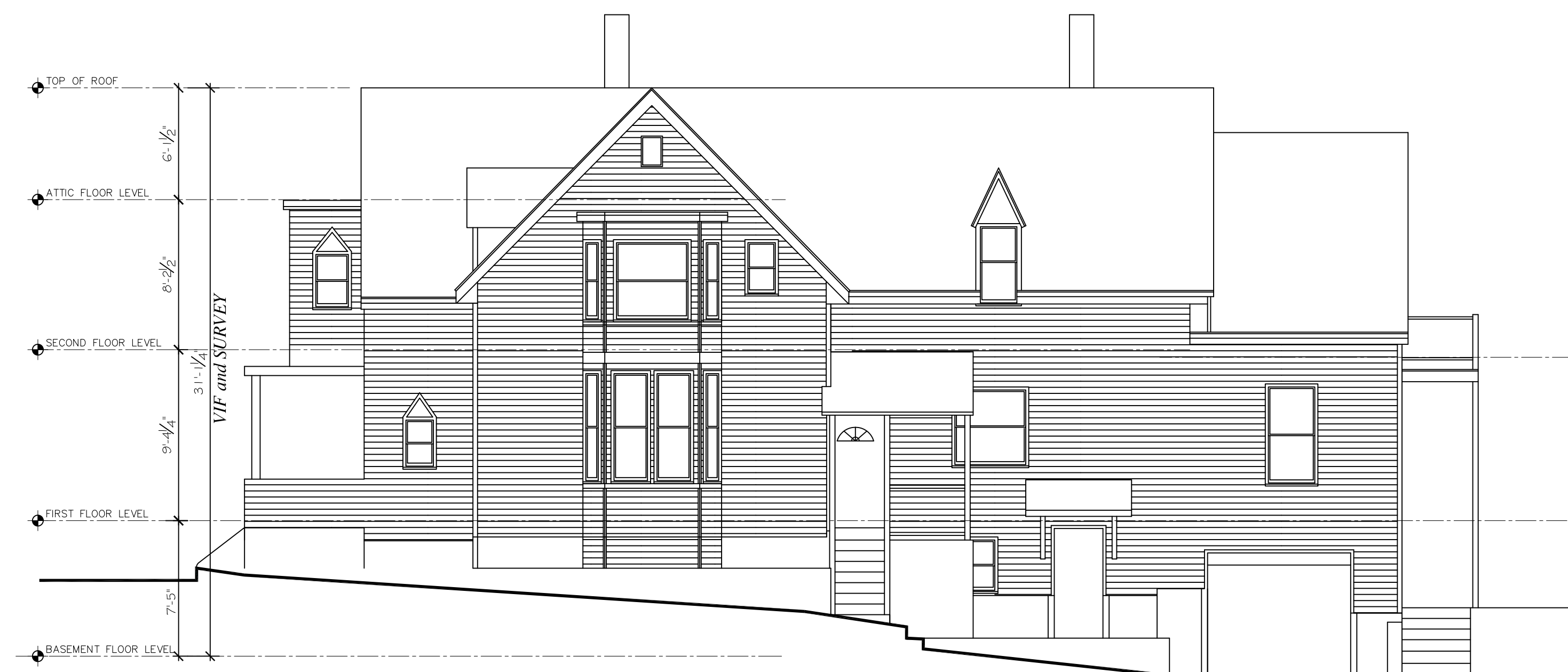
EXISTING RIGHT SIDE ELEVATION UNITS 1 & 2
