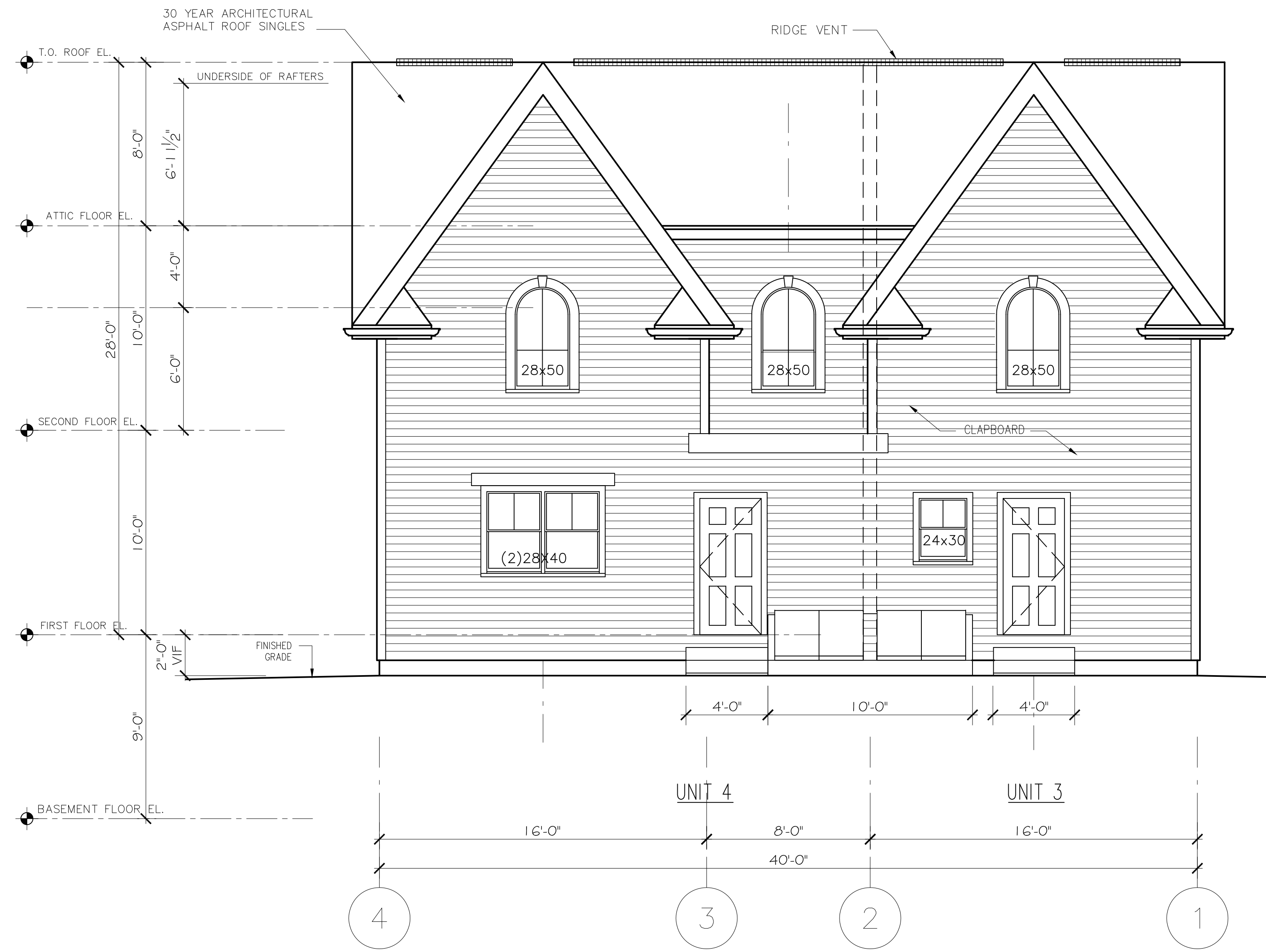
PROPOSED REAR ELEVATION UNITS 3&4
