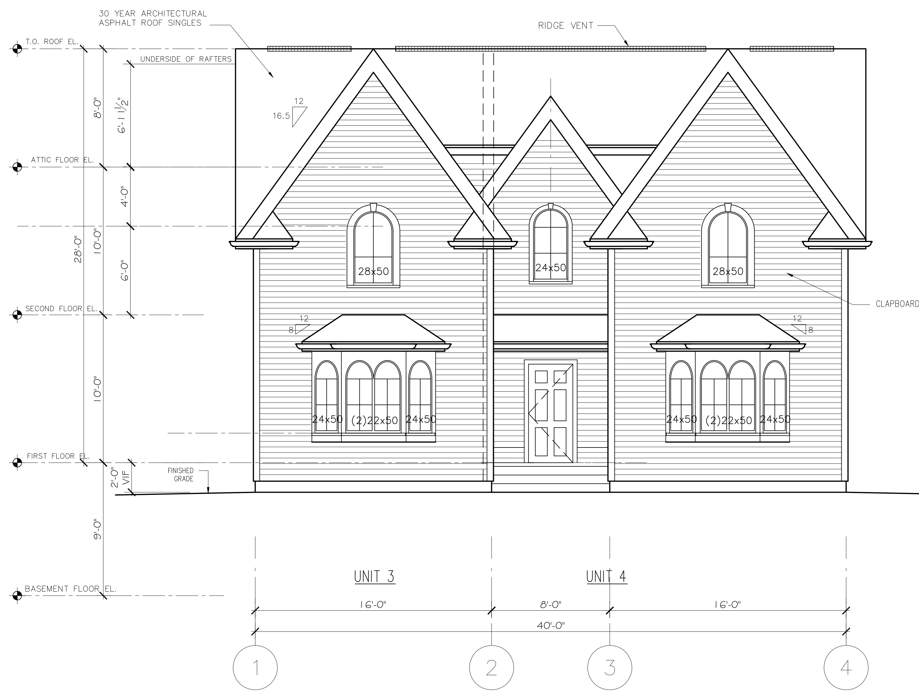
PROPOSED FRONT ELEVATION UNITS 3&4 SCALE: 1/4" = 1'-0"
