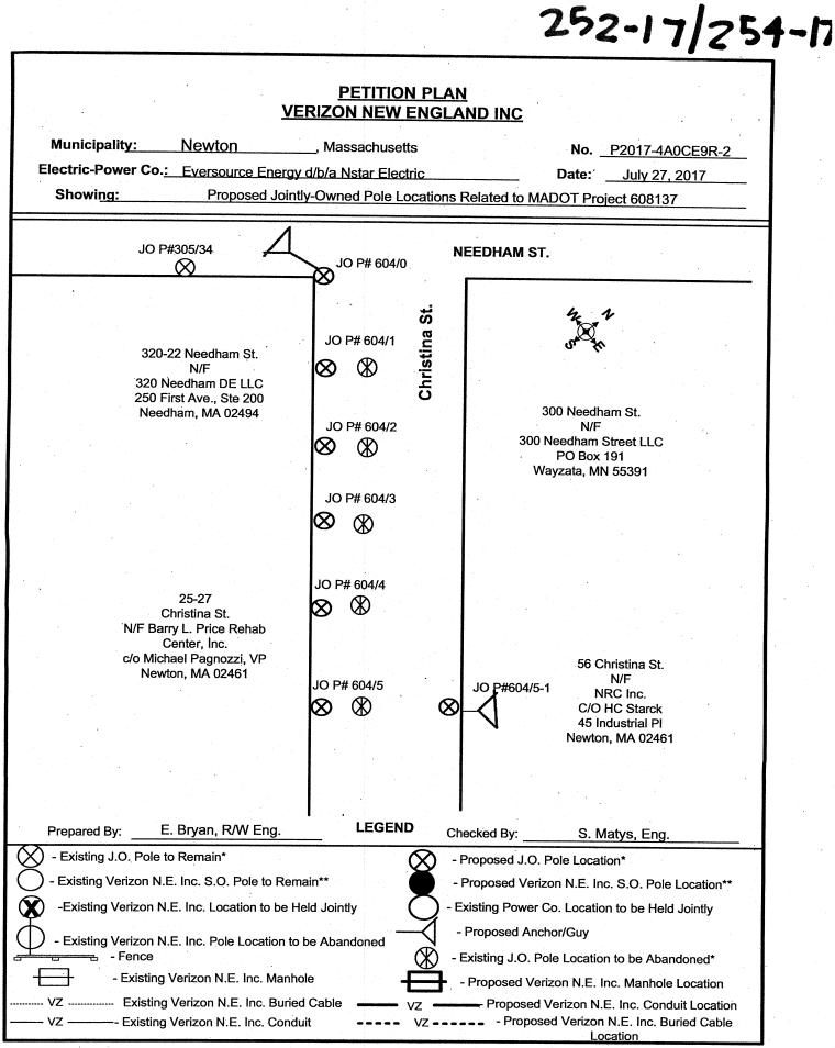
\*J.O. indicates Poles Jointly-Owned by Verizon N.E., Inc. & Power Co. \*\*S.O. indicates Poles Solely-Owned by Verizon N.E., Inc. or Power Co.
