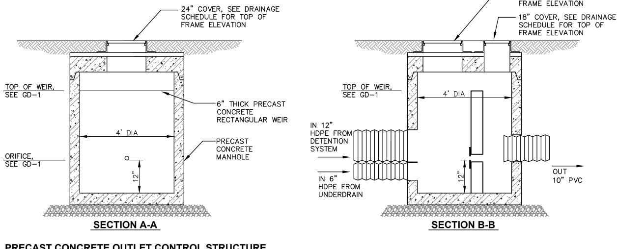
PRECAST CONCRETE OUTLET CONTROL STRUCTURE
