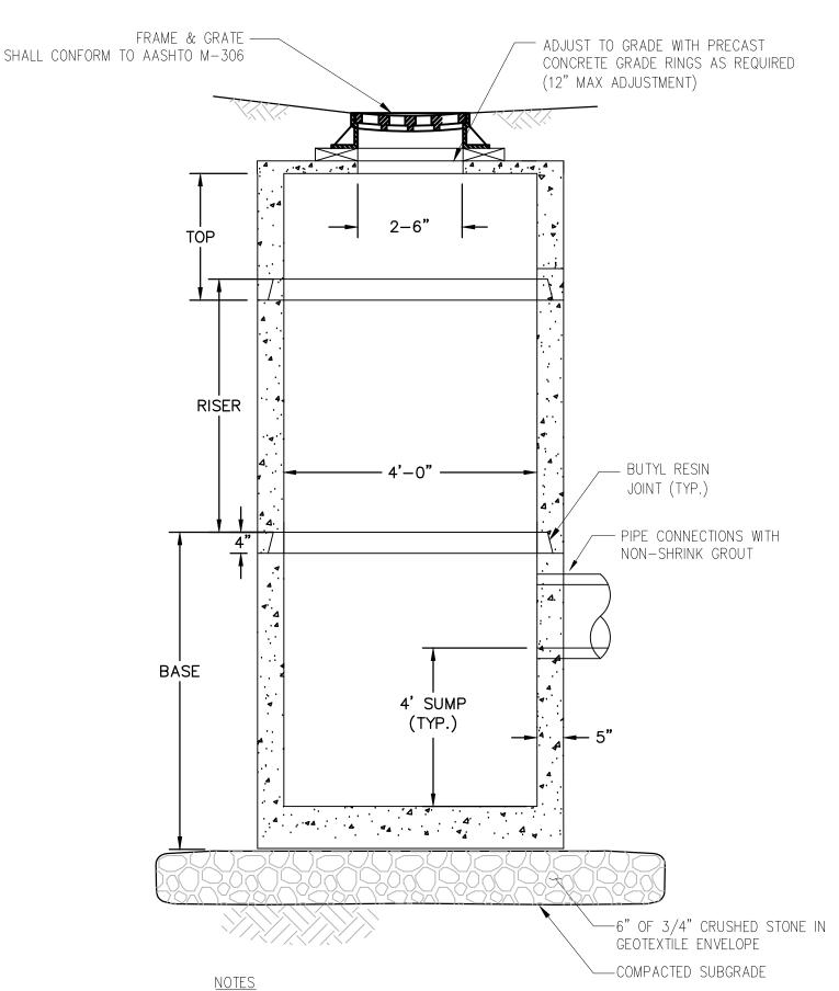
. CONCRETE: 5,000 PSI MINIMUM AFTER 28 DAYS. REINFORCED STEEL SHALL CONFORM TO LATEST ASTM A185 SPEC. 3. STRUCTURE PRECAST REINFORCED CONCRETE SHALL BE DESIGNED FOR H-20 LOADING PER AASHTO HS-20-44, AND IN ACCORDANCE WITH ASTM C478 SPEC FOR "PRECAST REINFORCED CONCRETE MANHOLE SECTIONS."
