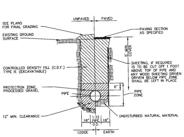
TYPICAL C.D.F. WATER TRENCH DETAIL NOT TO SCALE
