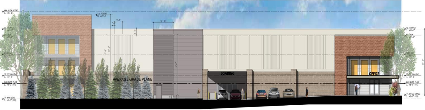
4 EXTERIOR ELEVATION - WEST - PARKING & ENTRANCE 1/8"=1'-0"
