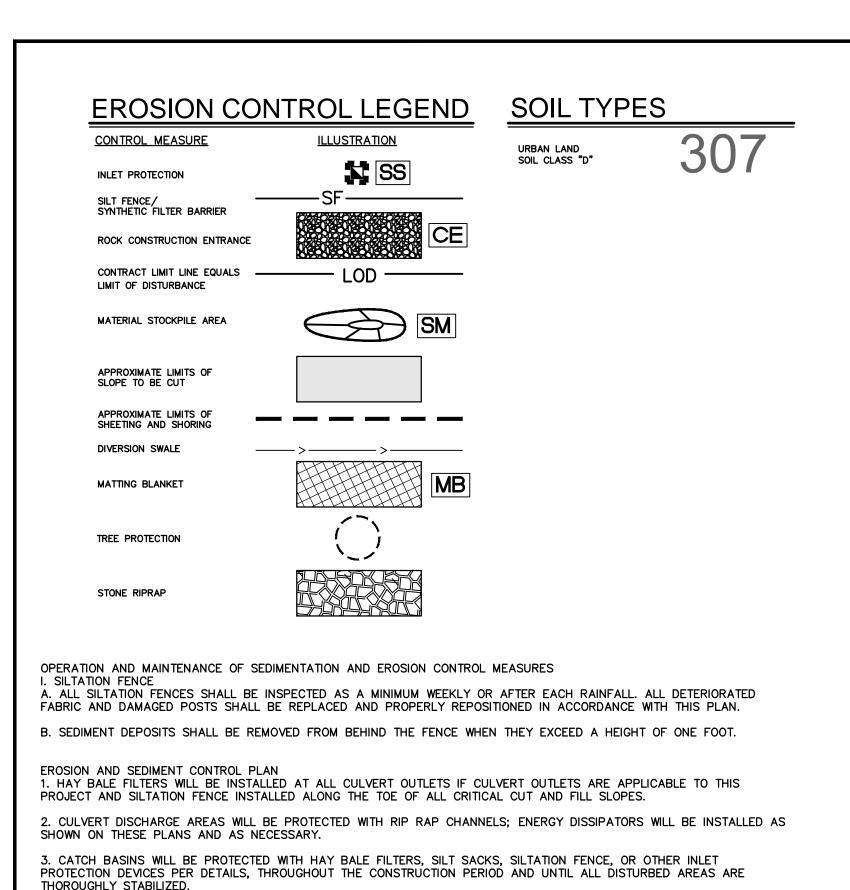
4. ALL EROSION AND SEDIMENT CONTROL MEASURES WILL BE INSTALLED IN ACCORDANCE WITH THE STANDARDS AND SPECIFICATIONS OF THE MASSACHUSETTS EROSION AND SEDIMENT CONTROL GUIDELINES FOR URBAN AND SUBURBAN
