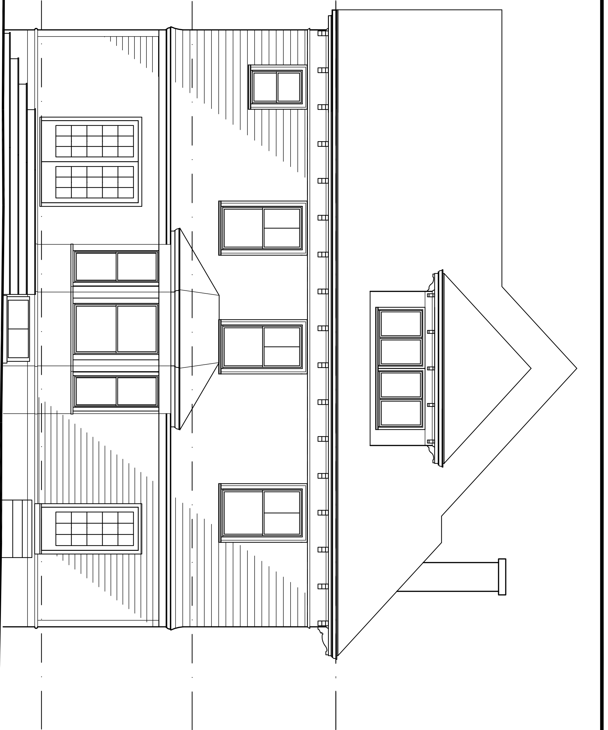
2 EXISTING REAR (WEST) ELEVATION 1/4"=1'-0"
