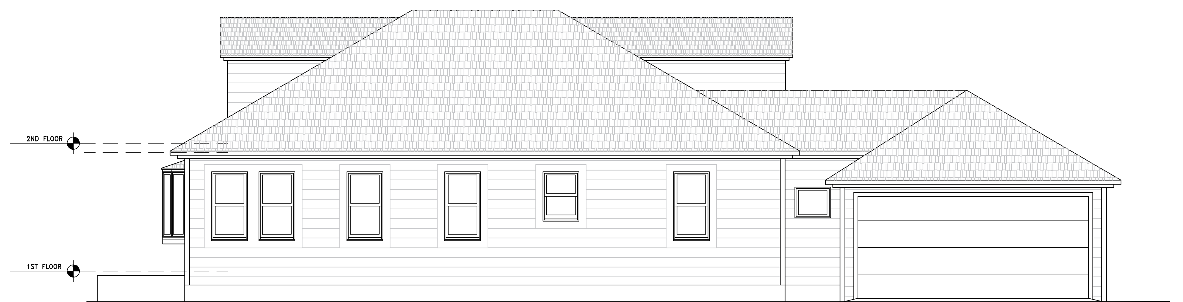
EXISTING REAR ELEVATION
