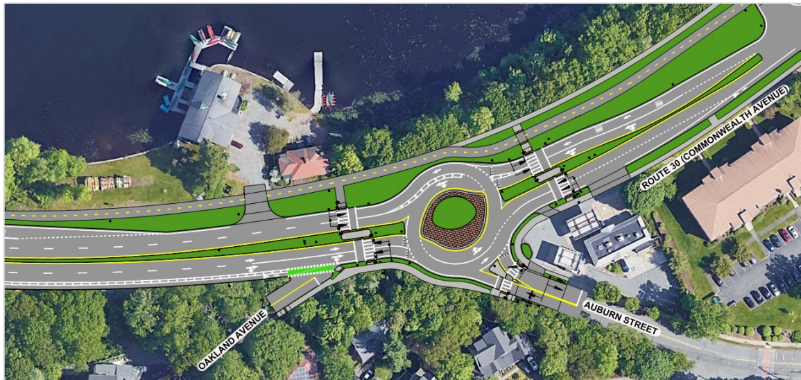
Figure 3. Mixed Lane Modern Roundabout Alternative
