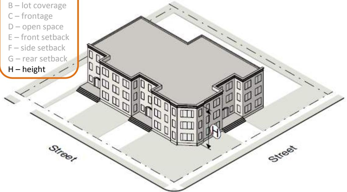
Dimensional Requirements control the dimensions of private property lots and the buildings constructed on them, including: width and depth of properties, height and overall scale or mass of buildings, as well as how far buildings are from the street and from neighboring property lines.
