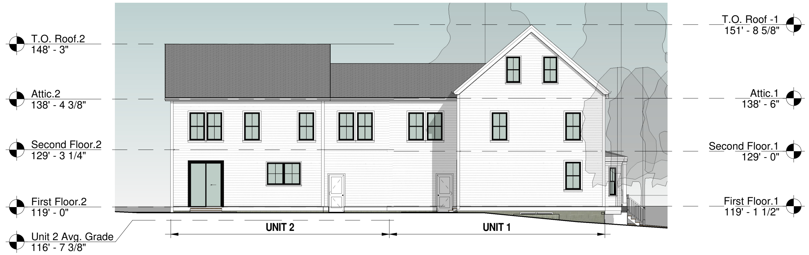
① Left Elevation Building 1 3/32" = 1'-0"
