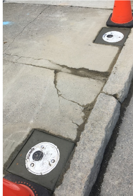
Conventional Drill Rig (top left) Geoprobe Drill Rig (bottom left) Monitoring Well Covers (above)
