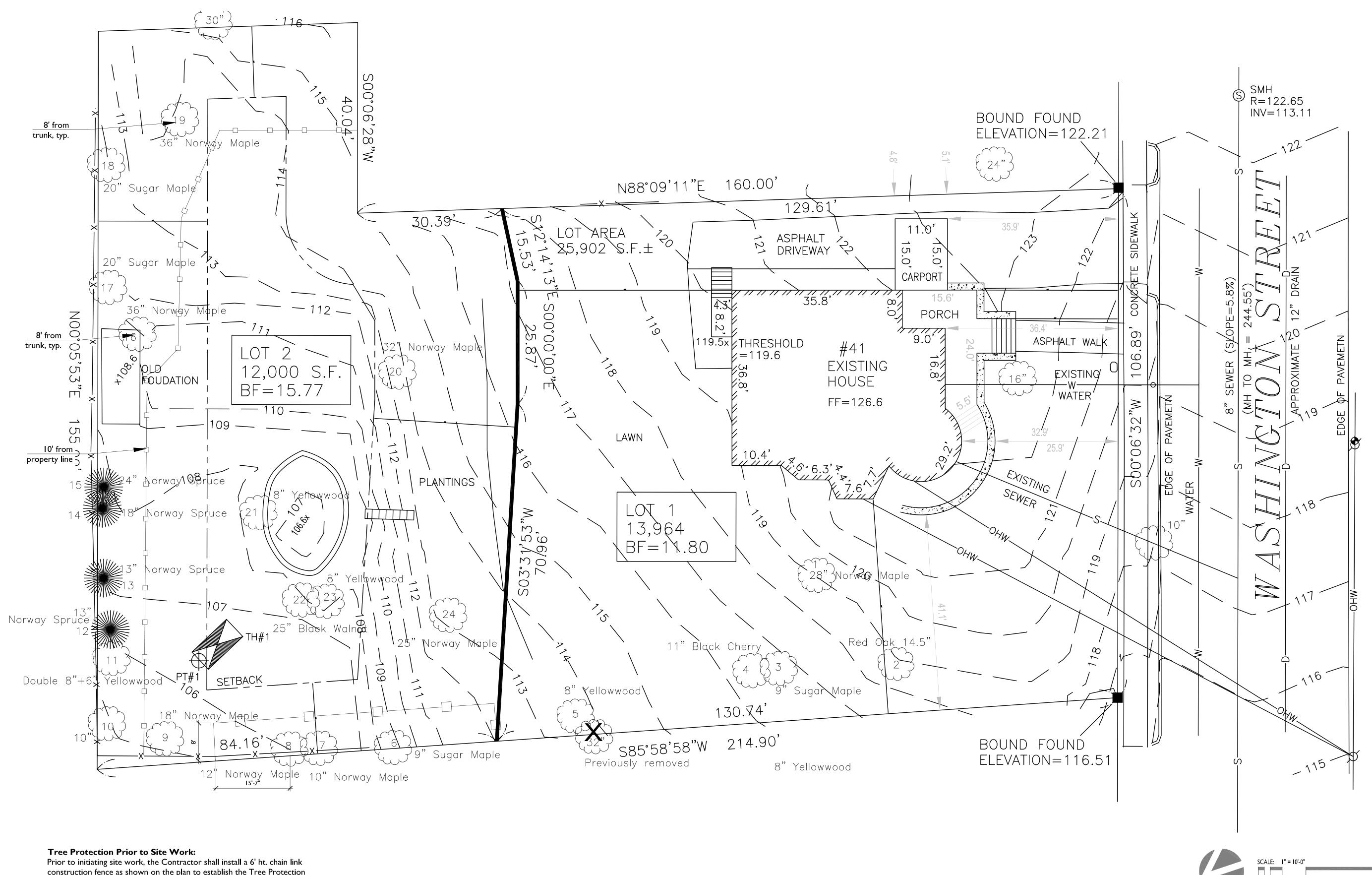
construction fence as shown on the plan to establish the Tree Protection Zone (TPZ). The Contractor shall not enter the tree protection zone with equipment, store equipment or materials within the TPZ for the duration of the construction project. The TPZ shall be maintained throughout the construction period and may only be removed as specifically directed by the Landscape Architect or Tree Warden.
