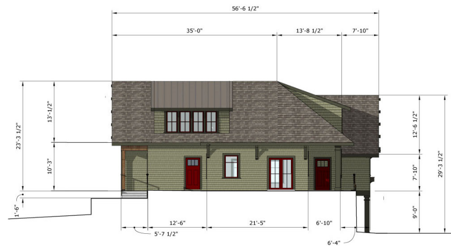
Front Elevation (Opposite Side-Raised Courtyard)
