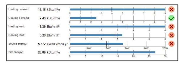
These results show the improvements from the baseline design simply by increasing the building airtightness from 0.31 cfm/ft² to 0.05 cfm/ft².
