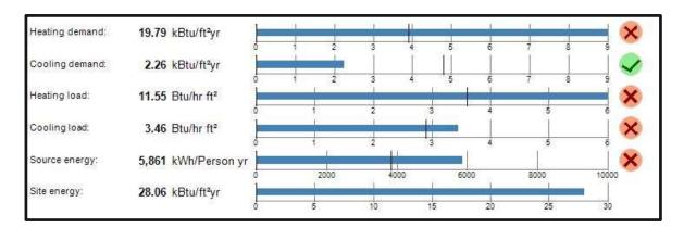
The initial baseline case shows the building fails to meet all Passive House thresholds but cooling demand. The reason cooling demand is easily met is due to higher air leakage and the northeastern climate.
