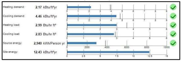
In order to meet the PHIUS requirements, the design would need to make adjustments to the building envelope and select high efficiency equipment for heating/cooling, ventilation and DHW. This also includes adding a 44 kW photovoltaic (60,000 kWh/year) system to the rooftop.
