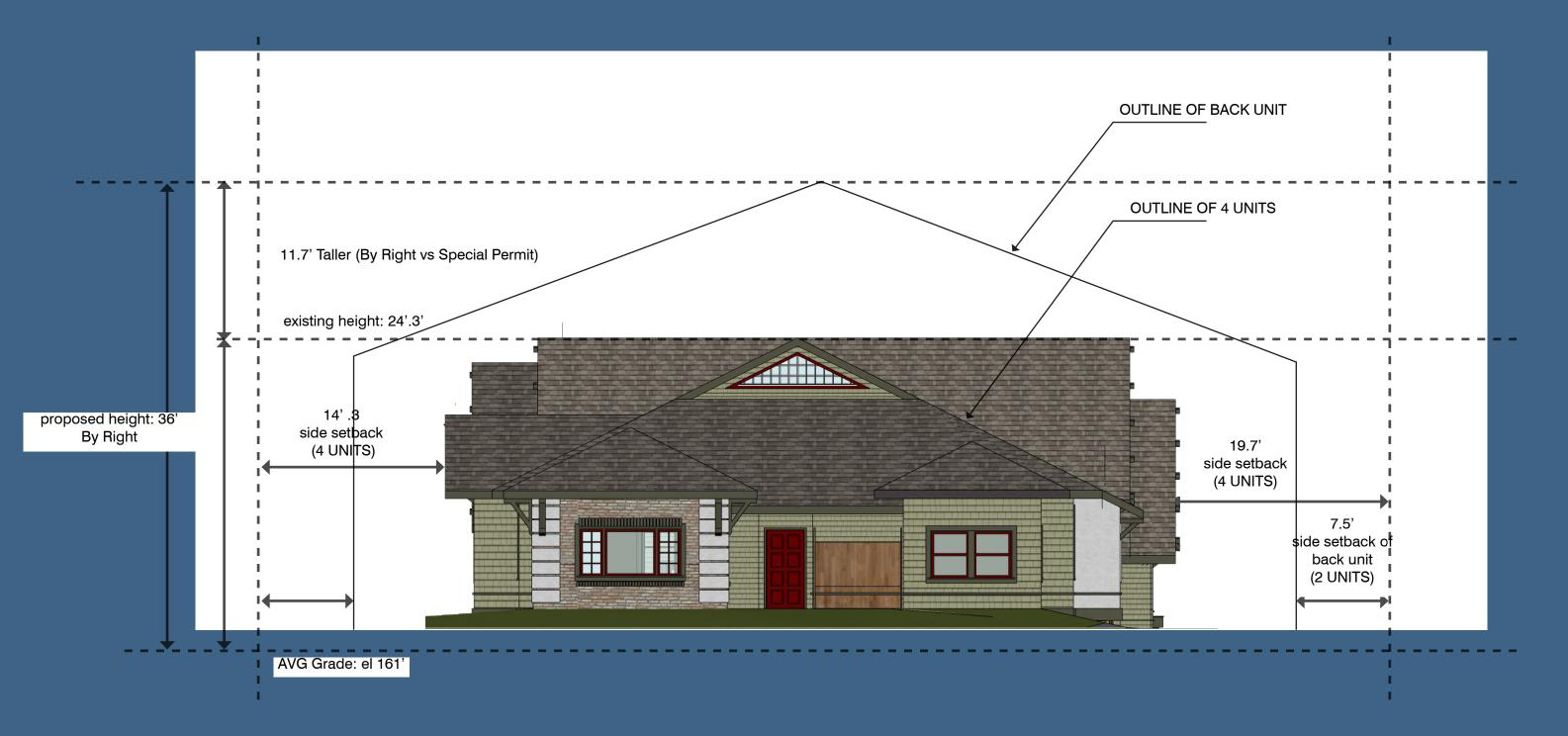
The by right option has significantly less side setback than the 4-unit design
