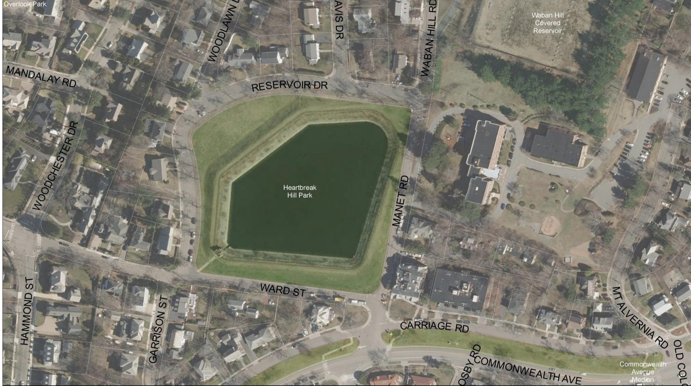
Heartbreak Hill Park @ Waban Hill Reservoir: 5-acre decommissioned open reservoir: 45% open water, 10% granite block wall, 10% walking path, 15% Steep grassy slope, and 15% somewhat-level area. 25% is usable space for recreational activity.
