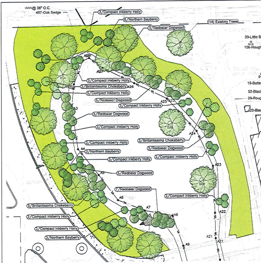
1 ENLARGEMENT PLAN 4 - EXISTING TREES, PROPOSED SHRUBS + GROUNDCOVERS SCALE: 1"=10'-0"
