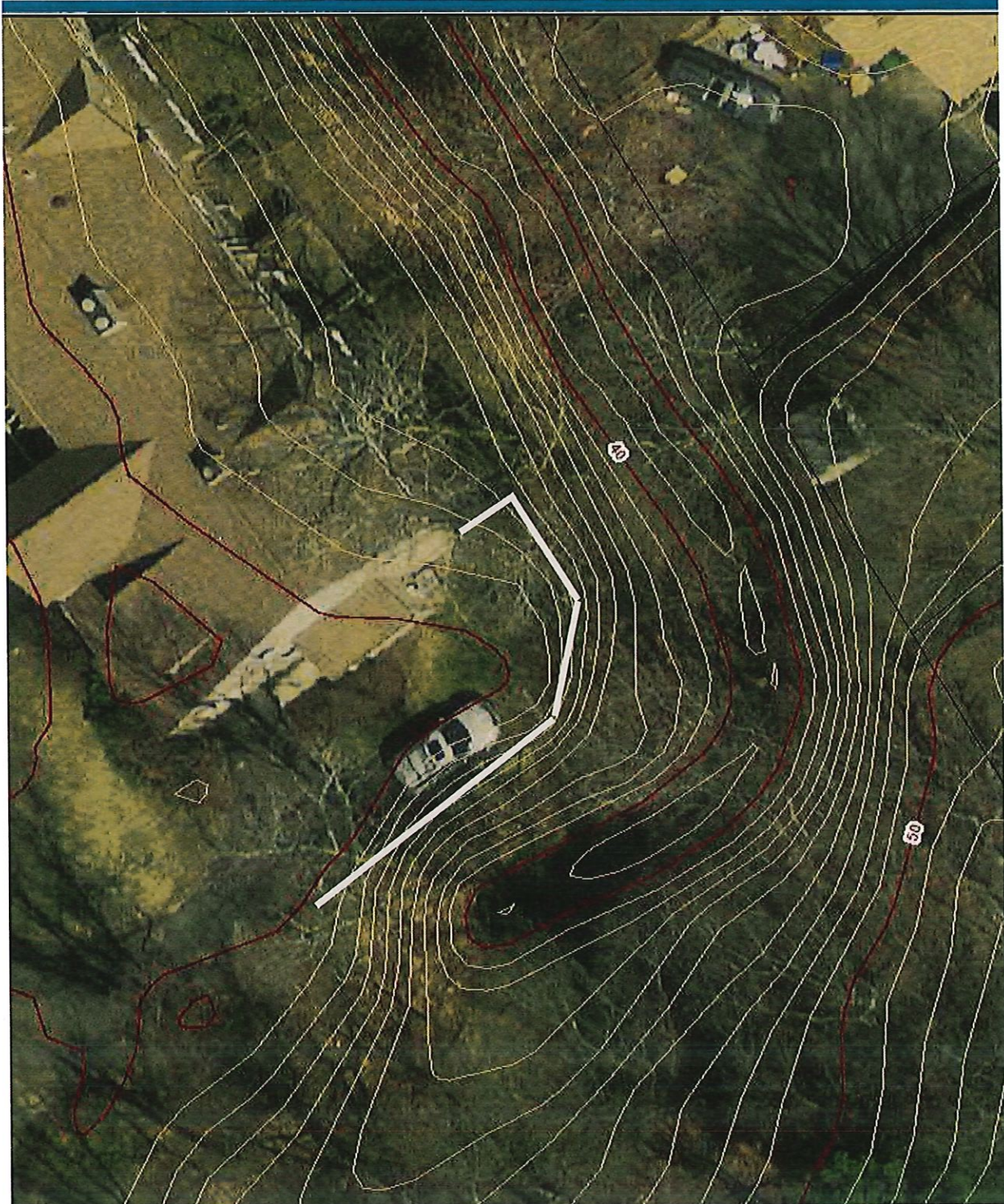
160 Pine Street aerial – illustration of retaining wall
