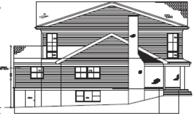
NORTH ELEVATION - NORTH (SIDE) SCALE: 1/8"=1'-0"
