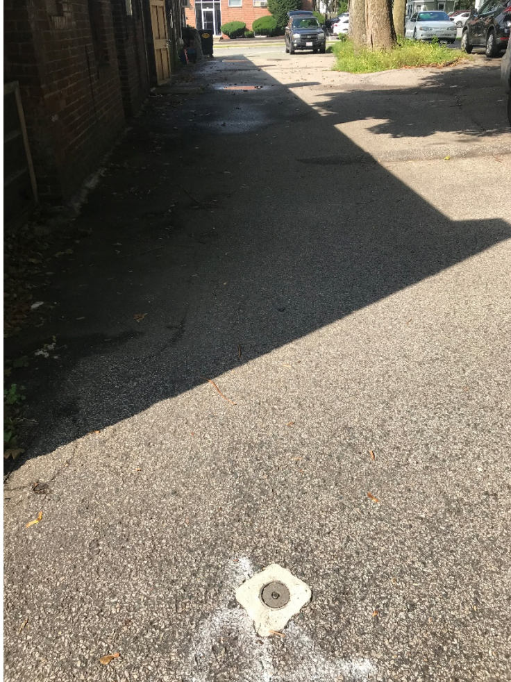
Monitoring Wellhead September 13, 2021
