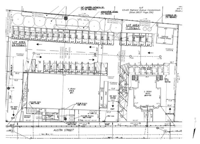
Also included within the revised site plan are enhancements to the front entrance such as an accessible ramp, concrete walkway, and increased bike parking.
