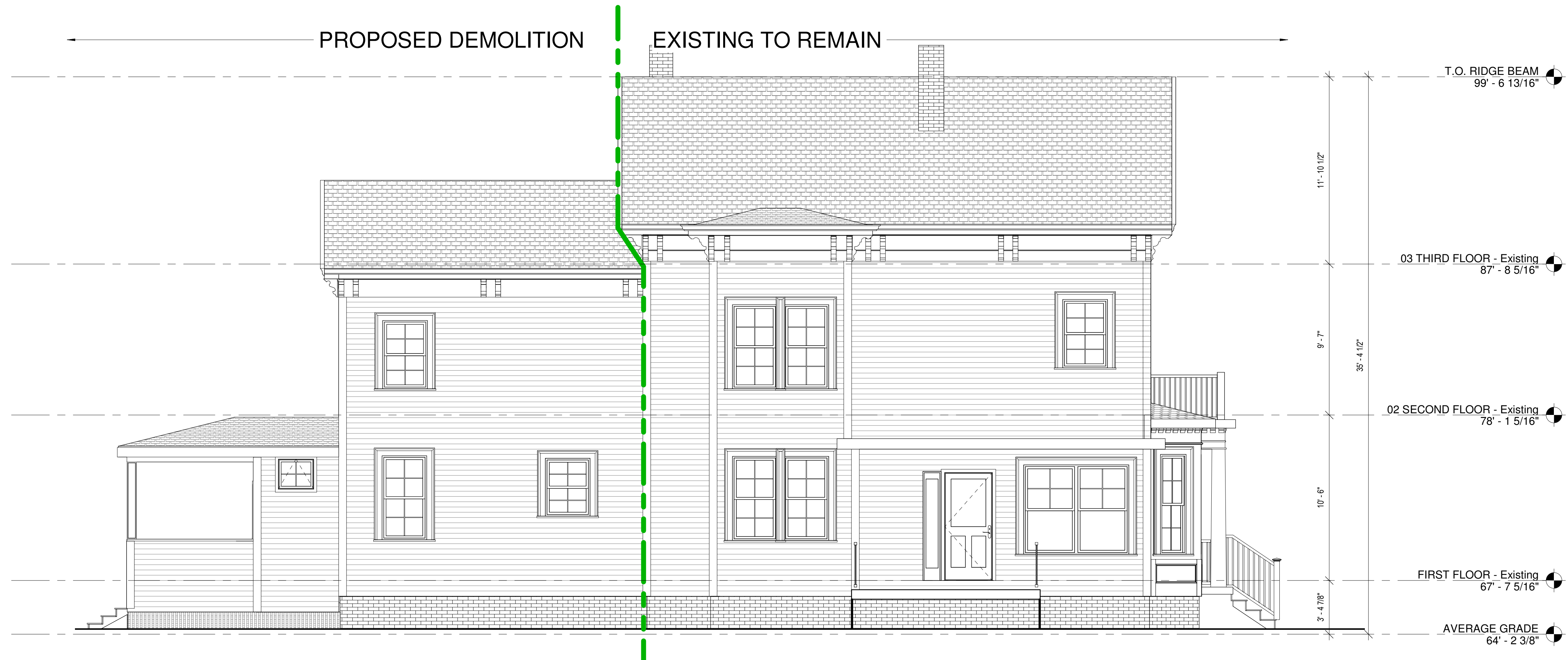
1 LEFT SIDE ELEVATION (EXISTING CONDITIONS) Scale: 1/4" = 1'-0"
