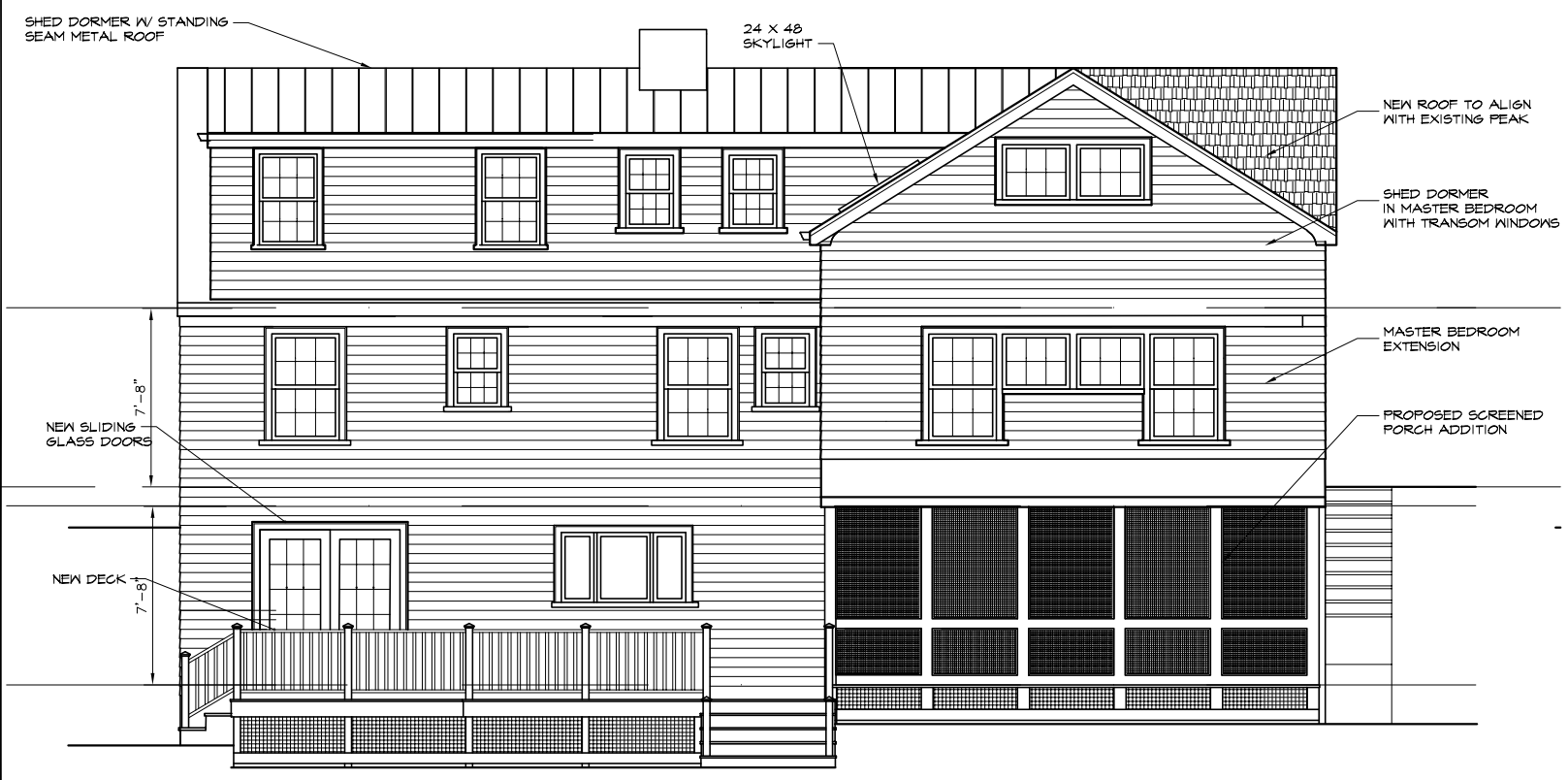
3 PROPOSED REAR NORTH ELEVATION A3 SCALE: 1/8" = 1'-0"
