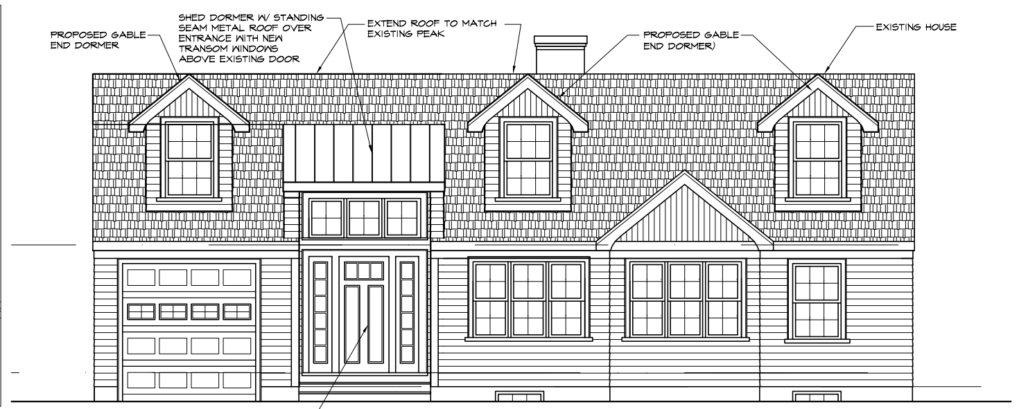
1 PROPOSED FRONT SOUTH ELEVATION A2 SCALE: 1/8" = 1'-0"
