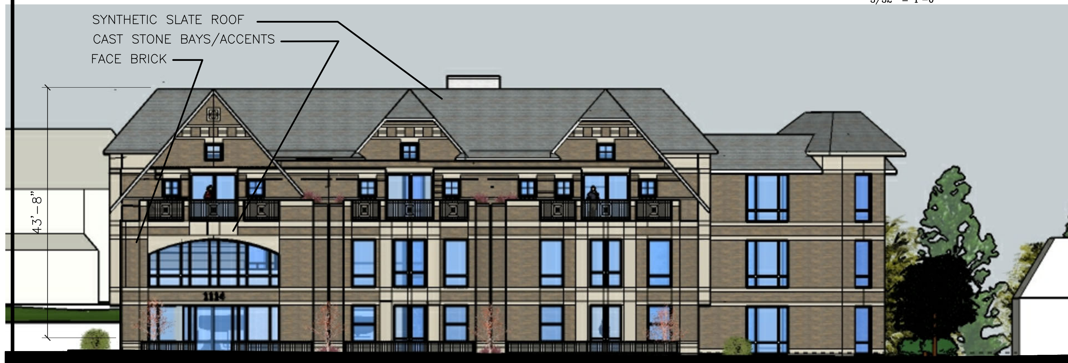
NORTH ELEVATION - BEACON STREET
