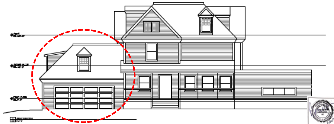
Proposed front elevation (new garage/addition indicated)
