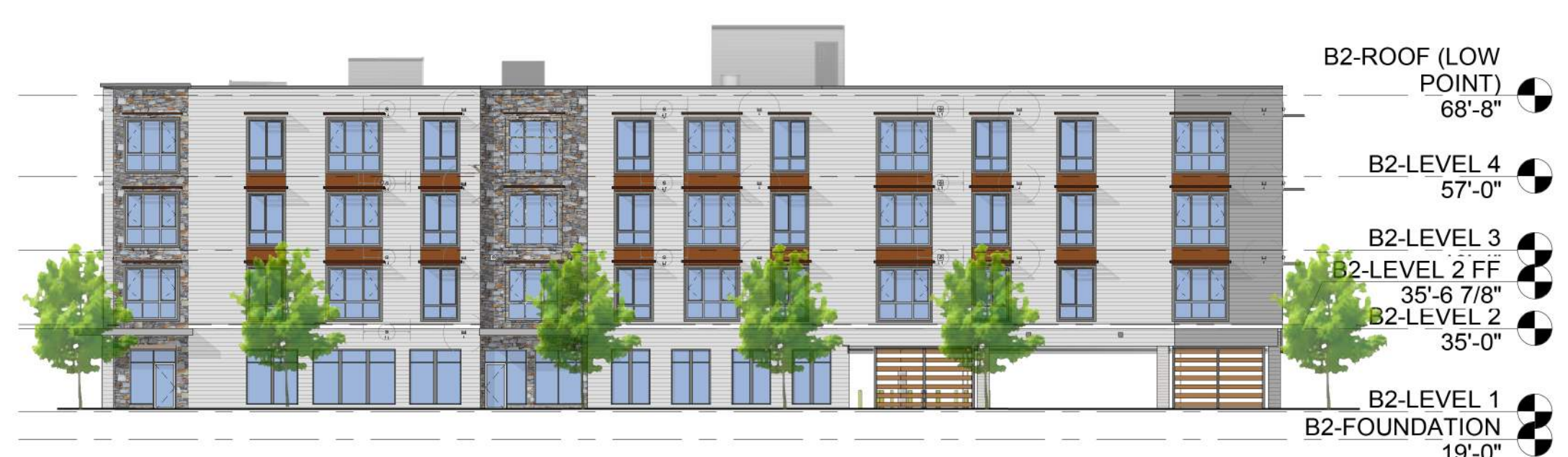
5 BUILDING 2 - WEST ELEVATION (LOS ANGELES STREET) 1" = 20'-0"
