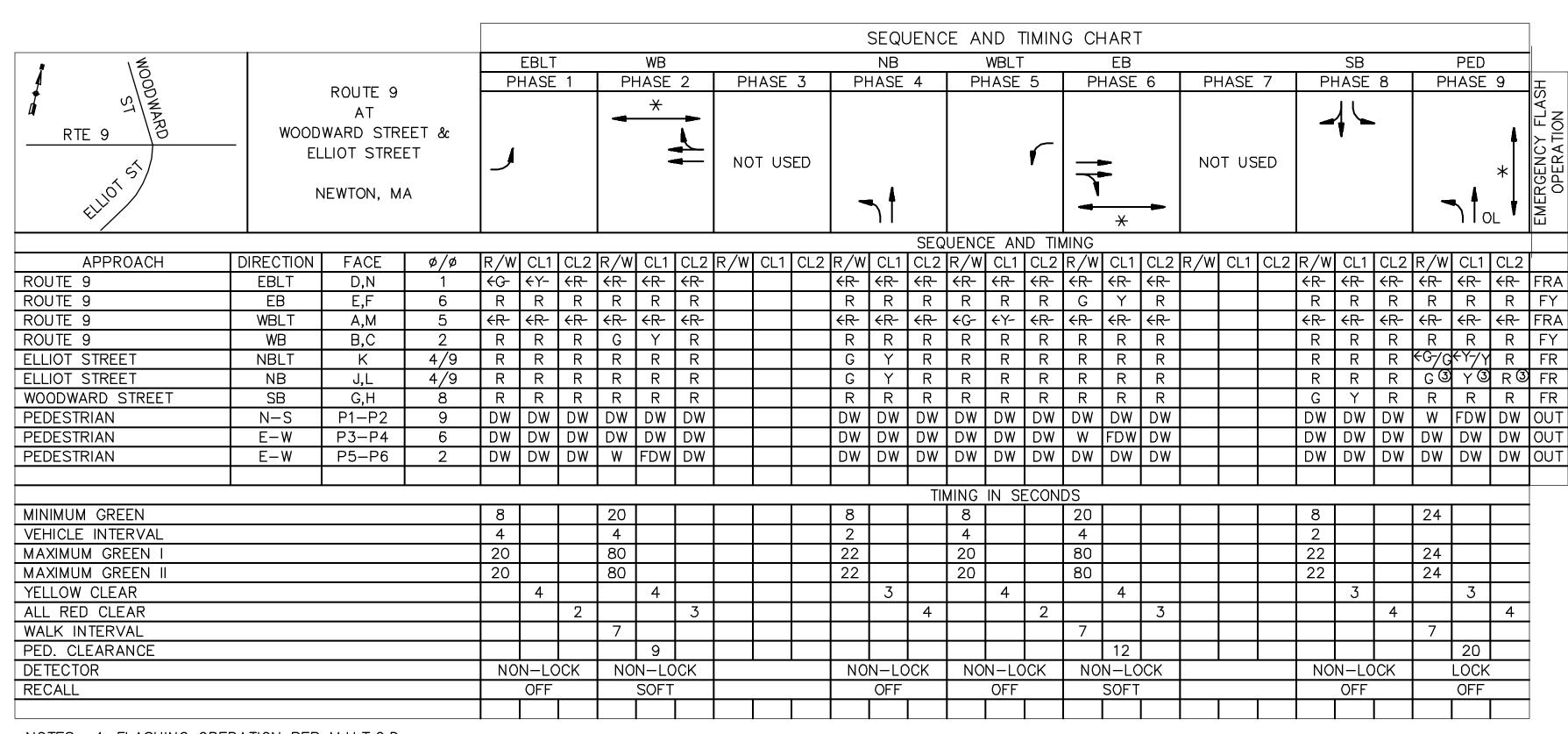
PROPOSED SIGNAL HEAD DATA A,D,M,NB,C,E,F,G,H,J,L P1-P6 16"x18" HOUSING 12" L.E.D. W/L.E.D. SIGNAL W/5" LOUVERED BACKPLATE INDICATIONS
