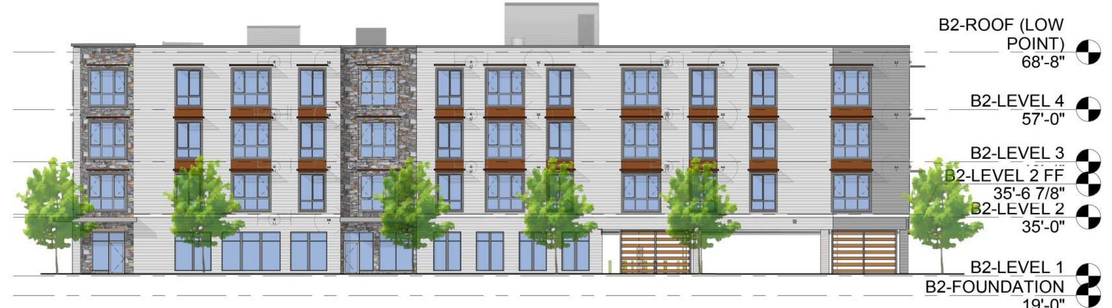
5 BUILDING 2 - WEST ELEVATION (LOS ANGELES STREET) 1" = 20'-0"
