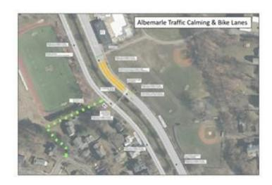
To improve safety, the project will slow down cars, add bike lanes, enhance crossings, and improve operations. The project uses quick-build and highly effective materials such as paint, flexposts and rubber speed cushions.
