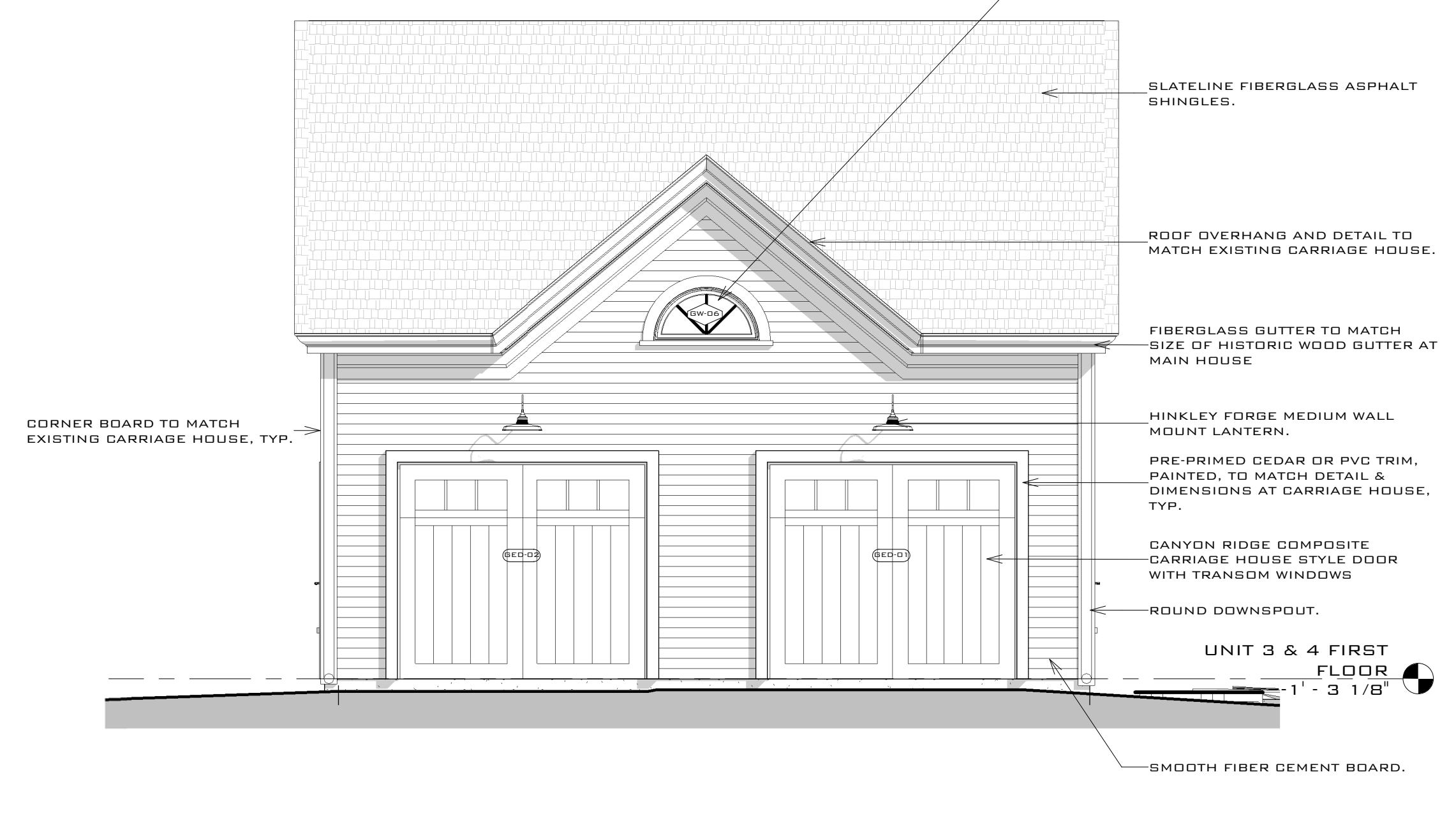
3 GARAGE FRONT ELEVATION 1/4" = 1'-0"
