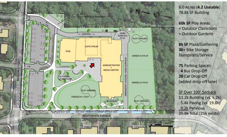
**SCHEMATIC DESIGN PROGRESS – SITE PLAN**
