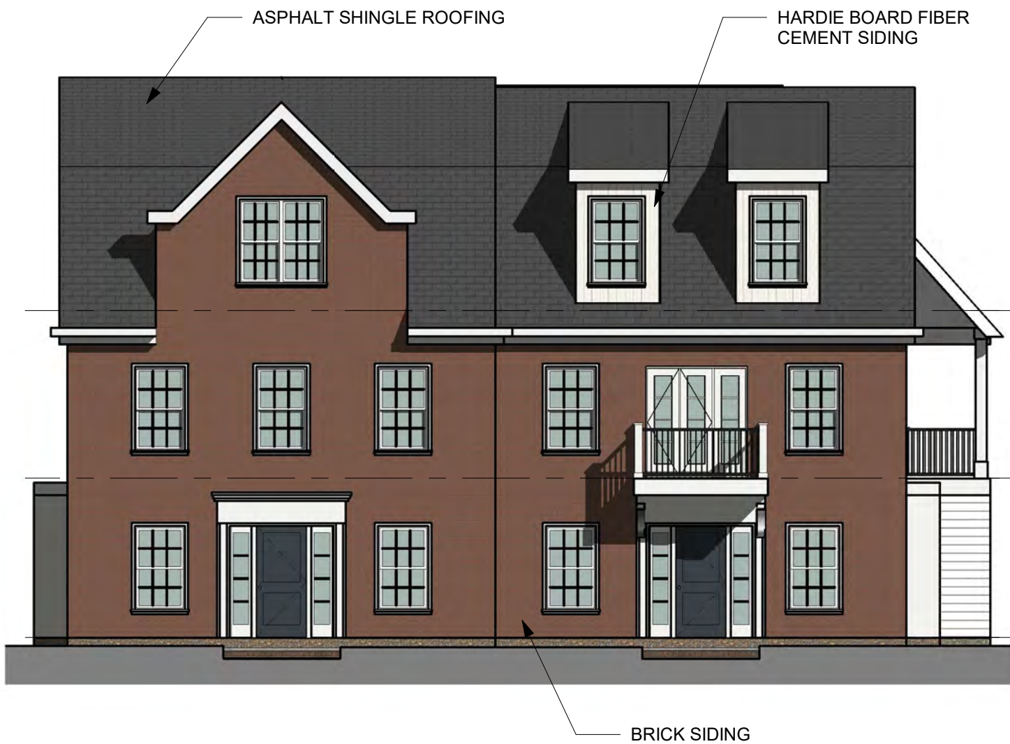
① BUILDING 1 FRONT ELEVATION 1/8" = 1'-0"
