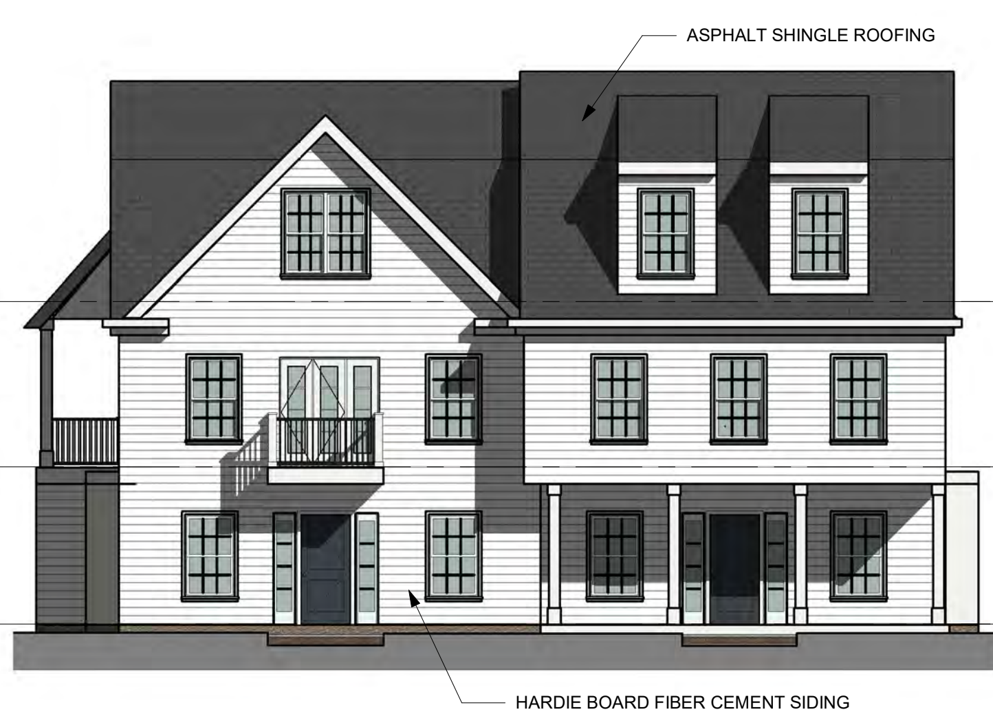
① BUILDING 2 FRONT ELEVATION 1/8" = 1'-0"
