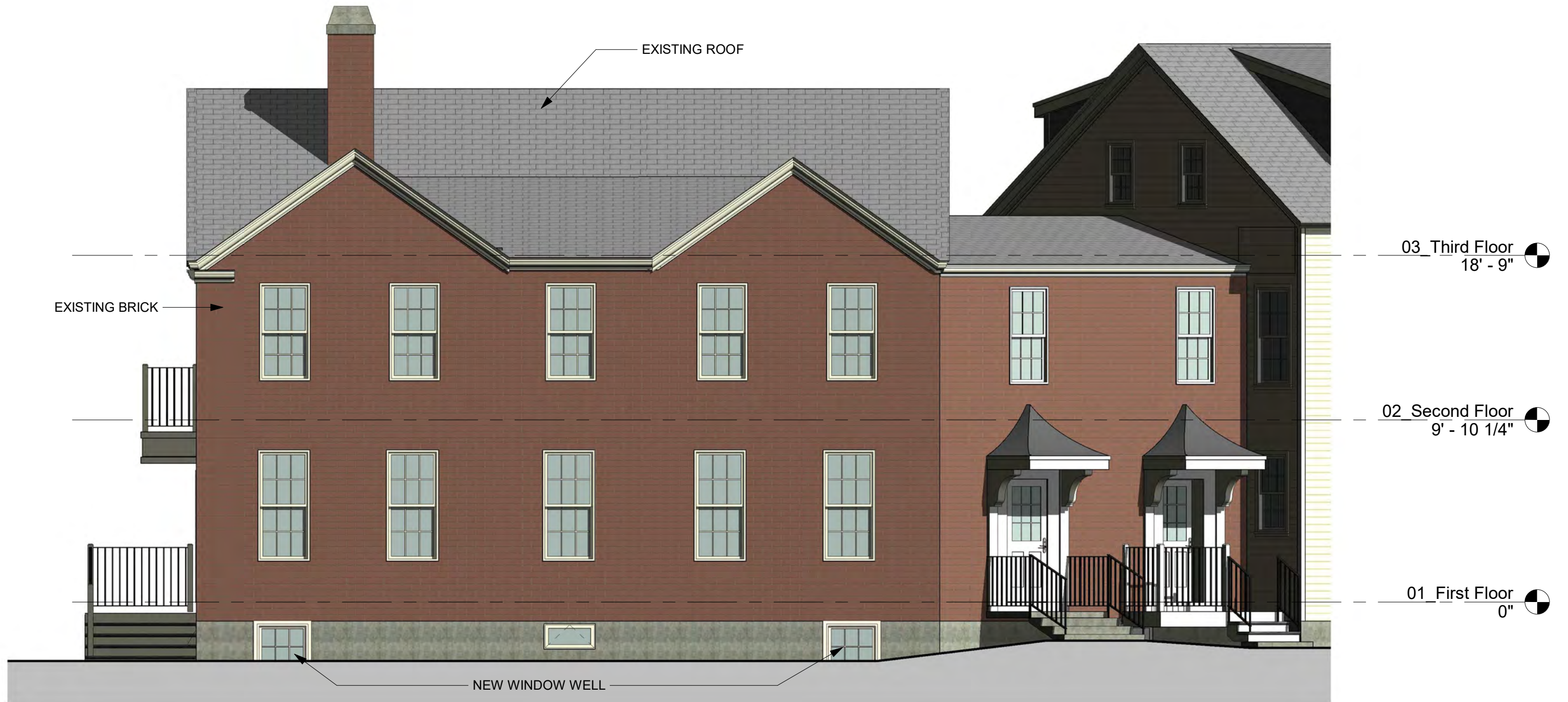
① Northeast Elevation 3/16" = 1'-0"
