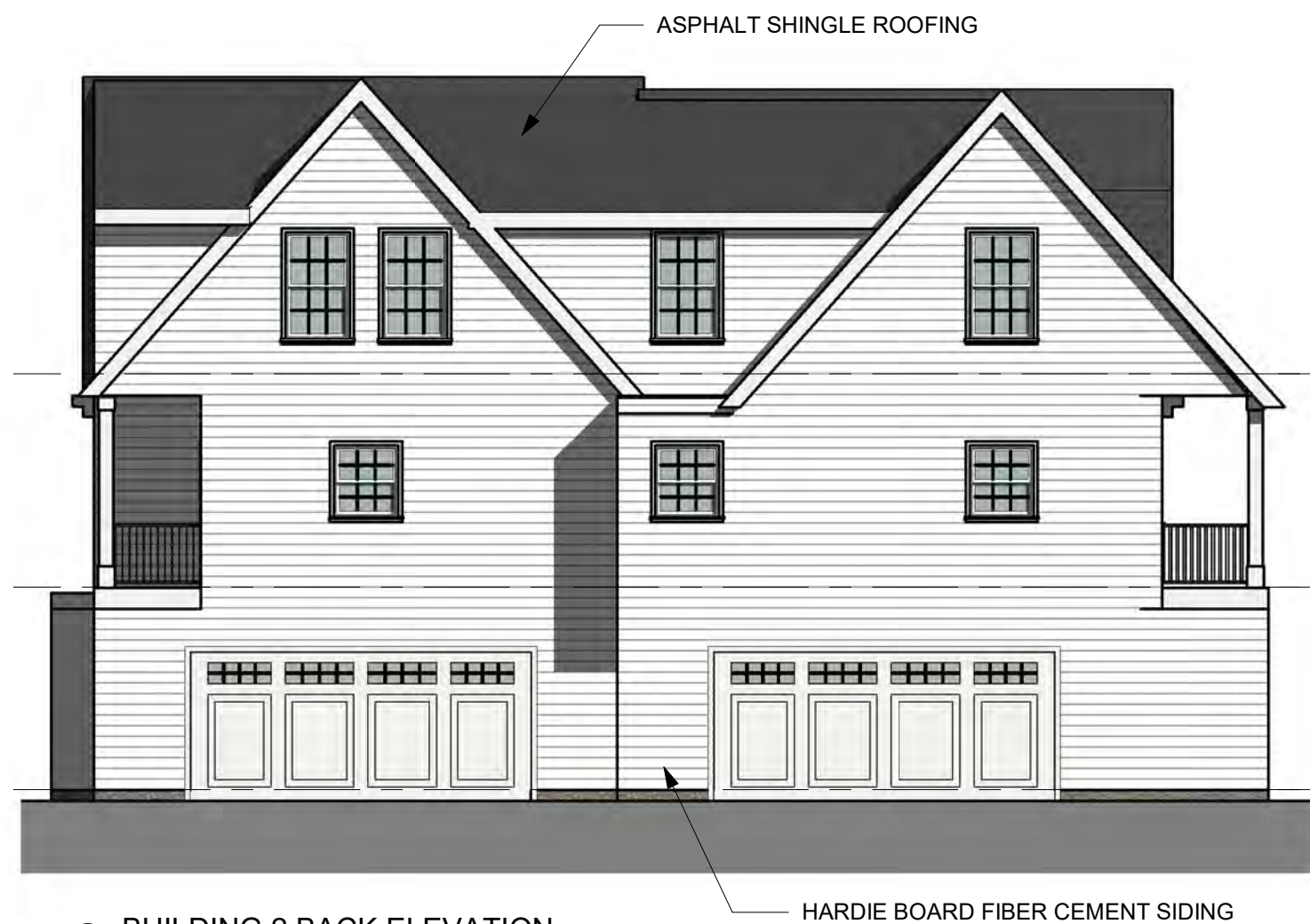
① BUILDING 2 BACK ELEVATION 1/8" = 1'-0"
