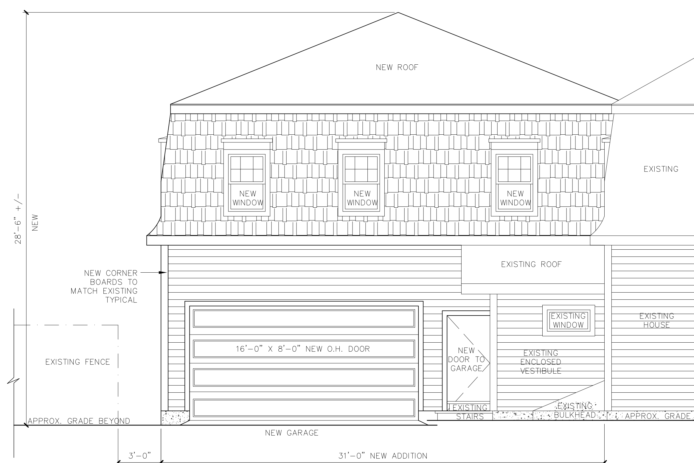
EXISTING RIGHT SIDE ELEVATION SHOWING PROPOSED ADDITION SCALE 1/4"=1'-0" ALL DIMENSIONS ARE +/- AND TO BE VERIFIED IN FIELD
