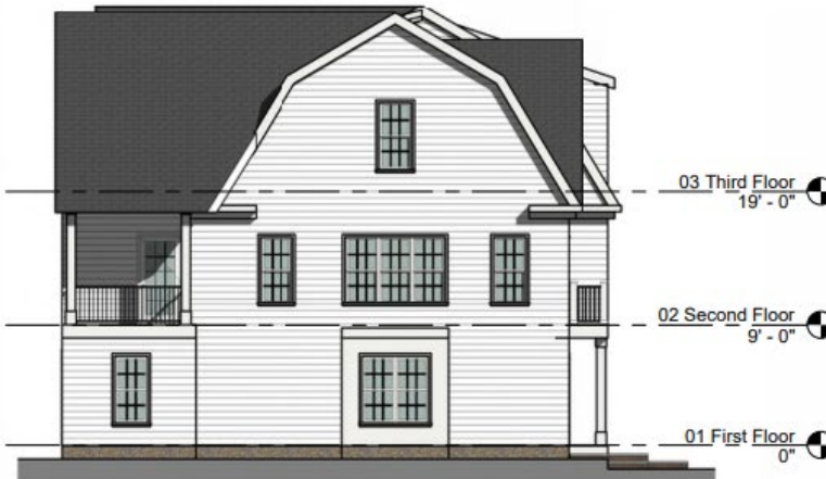
② BUILDING 2 LEFT SIDE ELEVATION 1/8" = 1'-0"
