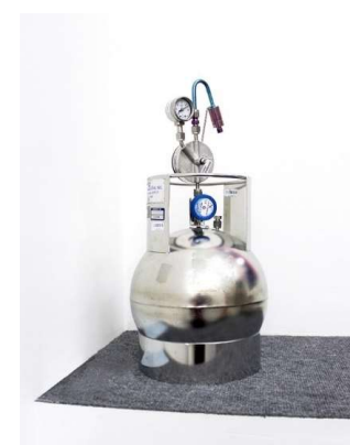
Installation and sampling of a sub-slab soil gas point (above) Canister for sampling indoor air (below)
