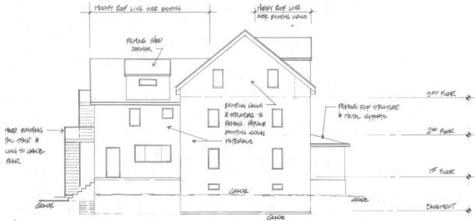
① LEFT SIDE ELEVATION - EXISTING 1/8" = 1'-0"
