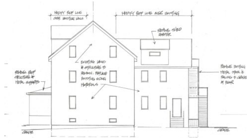
③ RIGHT SIDE ELEVATION - EXISTING 1/8" = 1'-0"
