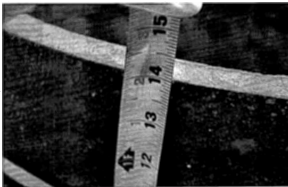
Figure 2: The pipe segment was 14-inches long.
